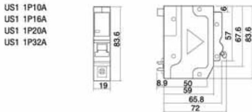
Figure 10 - 1 Pole Plug On Type Circuit Breaker
